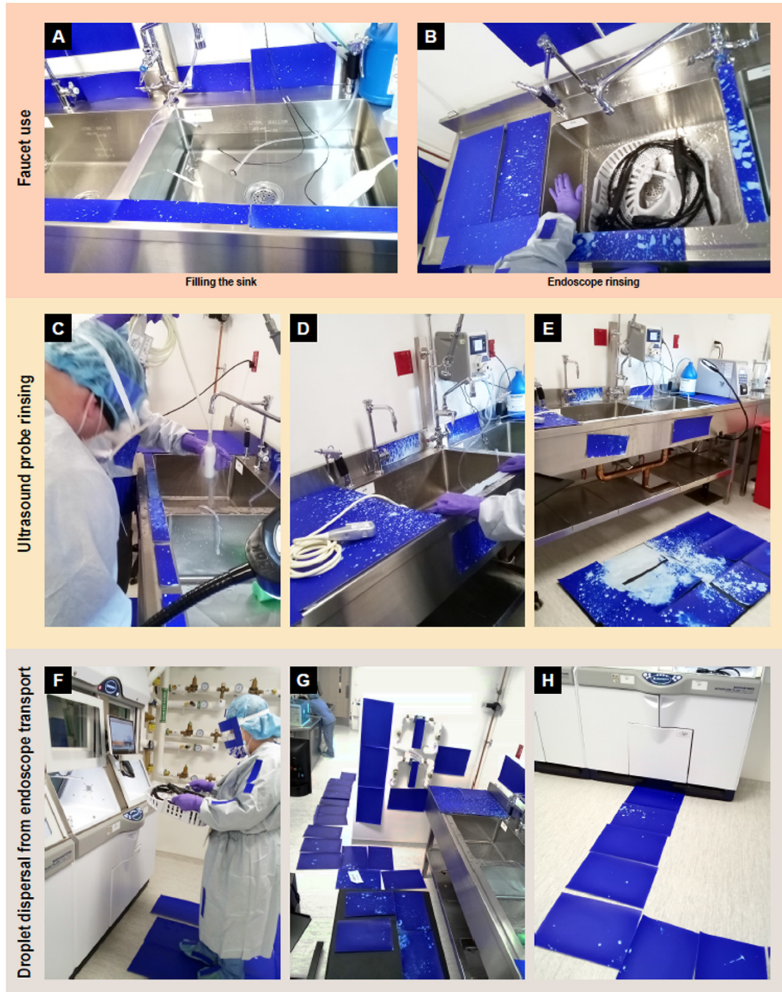
Fig 2. Workstation exposure to droplets during decontamination activities.
