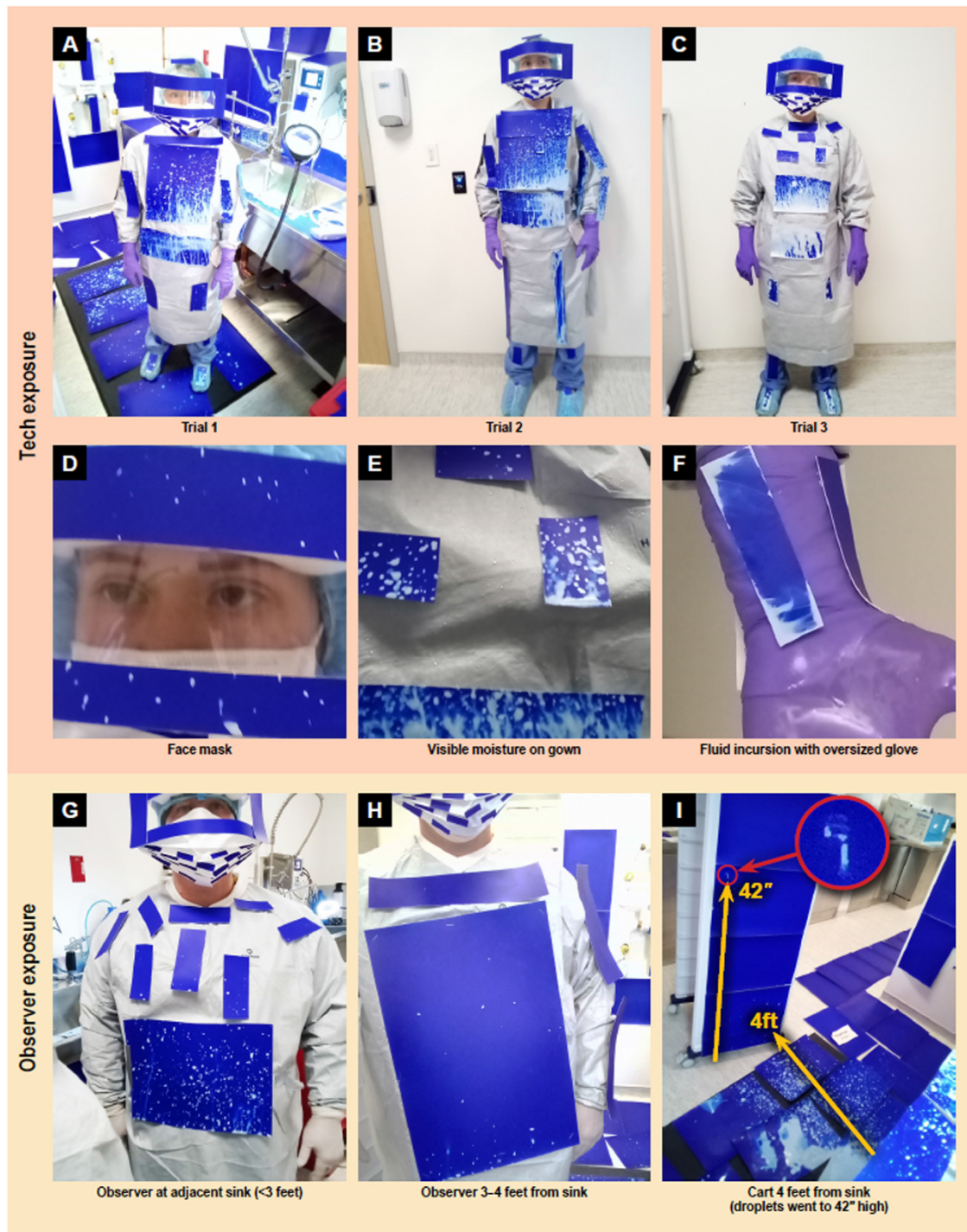
Fig 3. PPE exposure to droplets generated during probe decontamination activities.
